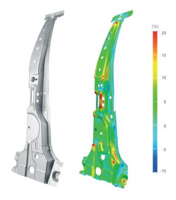
The optical forming analysis using ARGUS has become a proven tool for evaluating forming processes and verifying simulations. In particular, the precise, accurate and user-independent measuring procedure as well as the surface representation of deformation distributions strengthened the acceptance of this measuring technology. This unique possibility to measure complex sheet metal parts with a high scanning density opens up new aspects for the verification of forming simulations.
